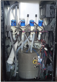
Step 1: Unplug the machine. Remove the back plate of your machine. Your machine hot tank will look like this.
